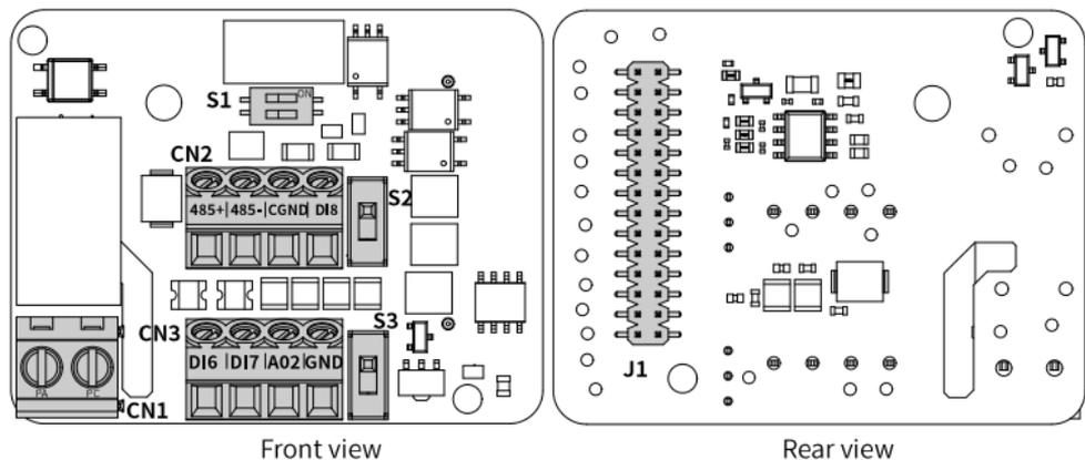
Figure 1-3 MD520IO1 card terminal layout
