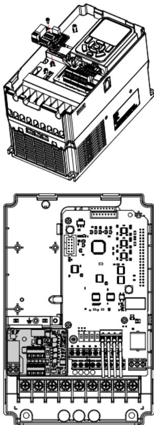
Figure 2-1 MD520IO1 card installation
