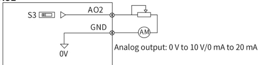
AO2: By default, the OFF state of the S3 DIP switch indicates the voltage mode with the output voltage ranging from 0 V to 10 V. The ON state of the S3 DIP switch indicates the current mode with the output current ranging from 0 mA to 20 mA.
